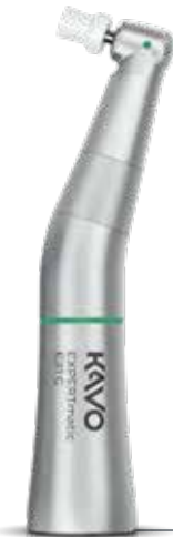
EXPERTmatic prophylaxis contra-angle E31 C (5.4:1, without light) Keeps out polishing paste thanks to multiple seals, with thread and knob, for screw-type and snap-on polishing attachments Mat. no. 1.008.4998
