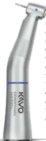
EXPERTmatic LUX speed-increasing contra-angle E25 L (1:5) Carbide guide bush, glass rod light conductor with up to 25,000 lux, fast, precise work thanks to small head, flexible latch and exclusive ceramic ball bearings, internally channelled spray water and spray air, CoolHead technology, 3-port spray and replaceable spray filter Mat. no. 1.007.5550
