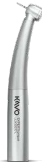
EXPERTtorque Mini LUX E677 L Small head: head height 12.2 mm, for standard and miniature burs, 27 watts of power*, 3-port spray, glass rod light conductor, up to 65 dB(A) (average 59 dB(A)) Mat. no. 1.007.3600
